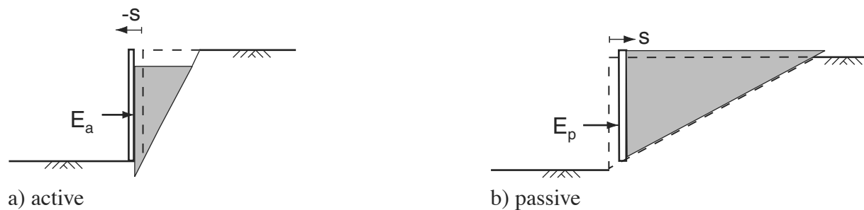
Figure 5.2: Active and passive earth pressures
